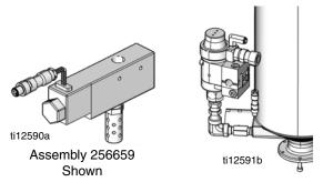
Assembly 256577 shown installed on tank for reference
